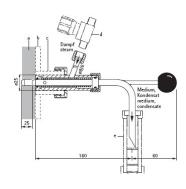
Sampling through the lid is achieved by the hypodermic needle technique using varied lengths of immersion tubes.
