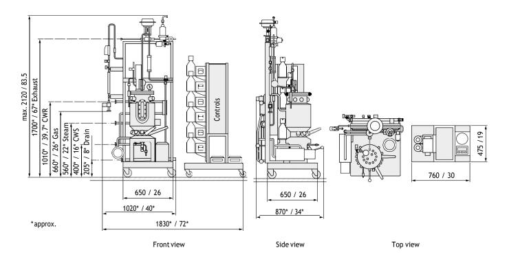
Dimensions are given in mm and inch and represent maximal values. Depending on fermentor configuration dimensions can be also smaller. White parts of drawing represent variable areas according to selected options.
